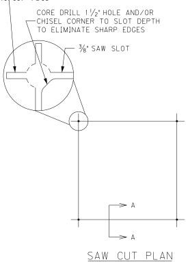
UNLESS SPECIFIED OTHERWISE, ALL LOOPS SHALL BE 6' x 6' SQUARE, CENTERED IN EACH LANE, WITH FOUR TURNS OF 14 AWG LOOP WIRE.
