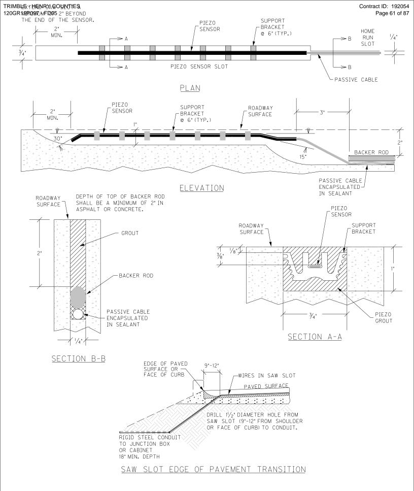
PIEZOELECTRIC SENSOR INSTALLATION
